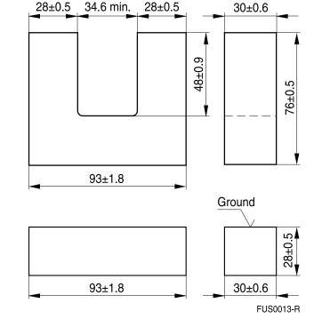
U and I cores are supplied as single units. The  $A_L$  value in the table applies to a core set comprising two ungapped cores.
